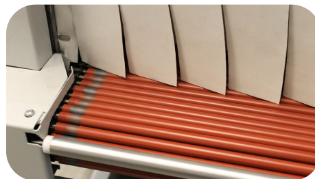
1" Roller spacing option for smaller products and when smoother product transfer is required
